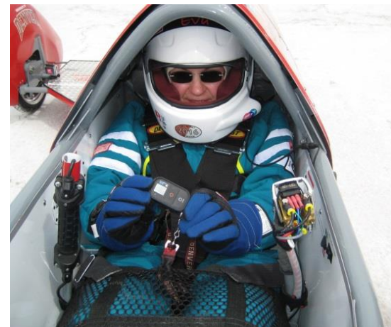
Your vehicle must be 100 % "race ready" in order to get an accurate estimate of the CG. That means that the driver is position and wearing all the safety equipment. Picture shows Eva in the KillaJoule electric sidecar streamliner.
